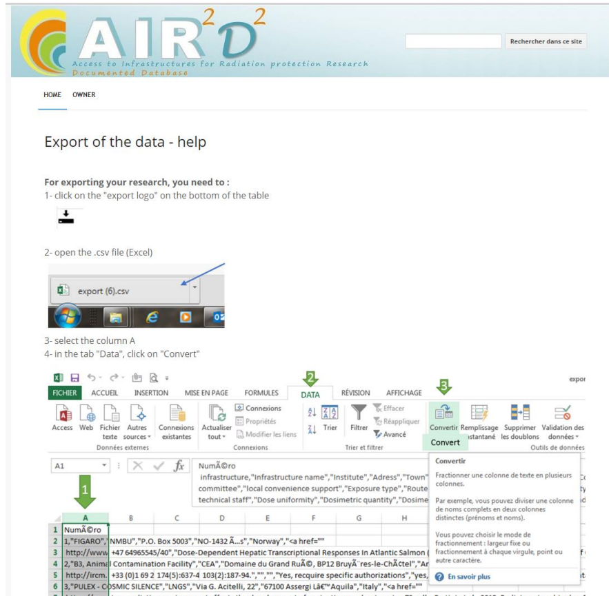
Figure 7: Tutorial on how to export and convert the data from an infrastructure search
